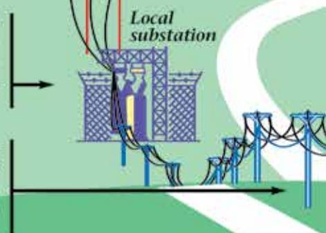
**Step 3.** Main distribution supply lines are checked next if the problem cannot be isolated at the substation. These supply lines carry electricity away from the substation to a group of consumers, such as a town or housing development. When power is restored at this stage, all consumers served by this supply line could see the lights come on, as long as there is no problem farther down the line.
